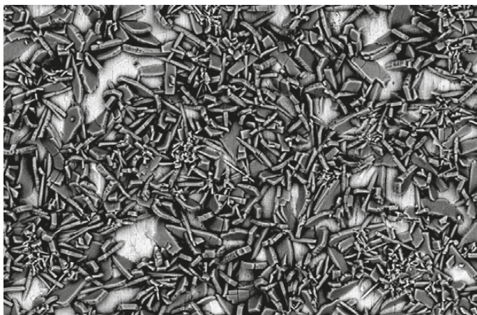
SEM image of Zinc-Phosphate on sheet metal
